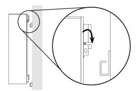
4 Insert the locking bar through the mounting bracket as shown.
