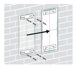
**3** Lift SolShare onto the mounting brackets as directed in the diagram. Check both top and bottom brackets are aligned and secured.
