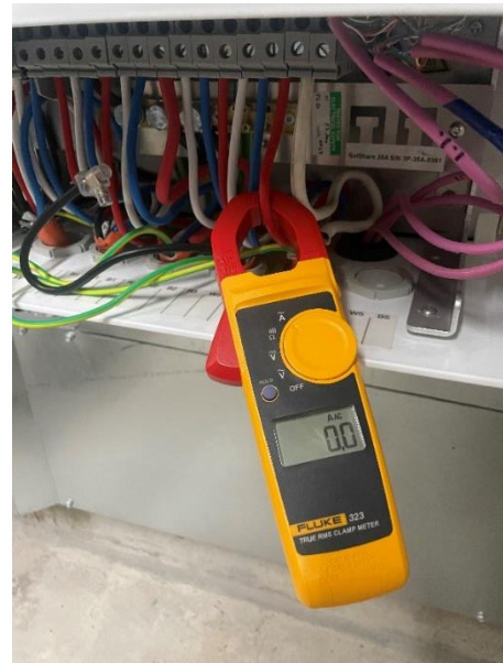
Fig 6. Test confirmation using a Clamp meter
