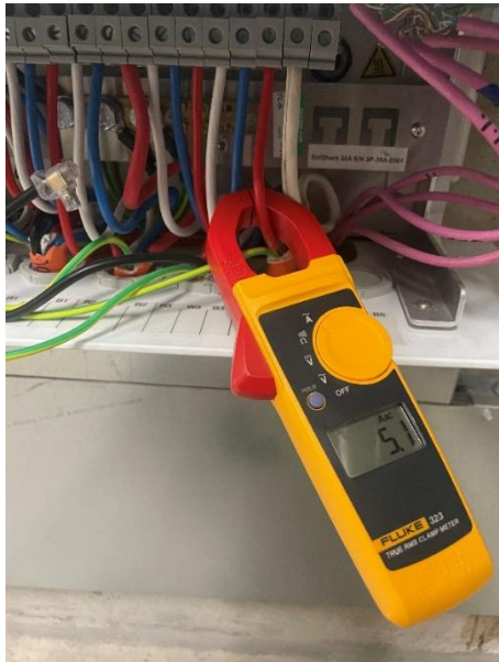
Fig 6. Test confirmation using a Clamp meter
